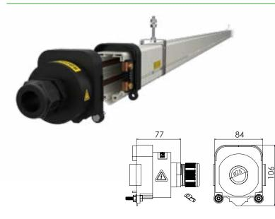
Designed for feeding the line at its end. In insulating material. Equipped with connection terminals and glands for round cable. Push-in tab and M6 nut-bolt (2 pieces) bar joint connection on bottom part.
